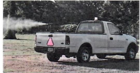
Photo courtesy of Ed Freytag, City of New Orleans Mosquito & Termite Control Board Mosquito control truck spraying insecticide into the air
